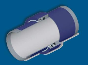
The ideal MIJ is one that is tested for a number of attributes before ever being installed. In this method, the chance of failure is greatly eliminated. Testing for the welds, the coating, electrical isolation, hydro-testing and pneumatic testing should all be done on each individual MIJ. The MIJ should have the same pressure class rating as a flange in the same pipeline and no part of the MIJ should protrude into the media stream.
