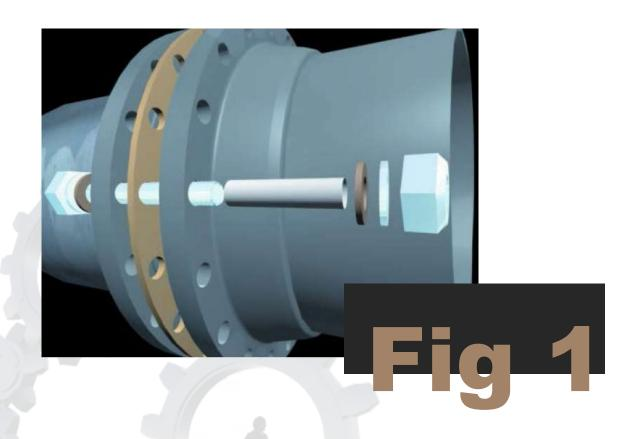
So Flange Isolation Kits have been around for a very long time and over the years we at GPT have modified designs and material selections in order that these kits can electrically isolate flanges conveying aggressive and sour media in critical service applications.
