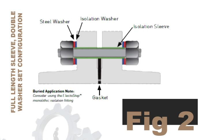
The typical make up of a standard non-fire safe FIK's is shown in fig 2. So in the event of a fire in a plant which spreads to the flanges, the two isolation washers which are located on both sides flange will burn away. These are 3mm thick, thus allowing the flanges to relax and open by 6mm allowing flammable liquid or gases to leak and fuel the fire.
