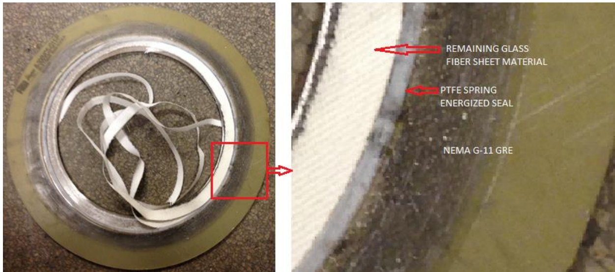
Figure 1: Shown is a GPT VCS™ gasket with SS316L core and NEMA G-11 GRE (green/yellow color) after being exposed to a steam based media for a few months. The glass fiber layers (white color) are all that remain between the PTFE seal (translucent white color) and the pipe bore/media after the epoxy was leached out during the chemical attack on the gasket. The gray color area is graphite residue from a previously installed spiral wound gasket in the flange assembly.
