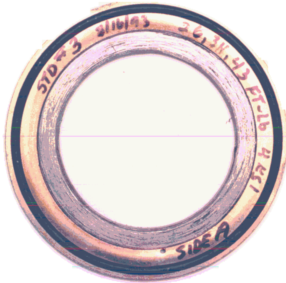
SPIRAL WOUND GASKET AFTER NITROGEN PRESSURE TEST SIDE A
