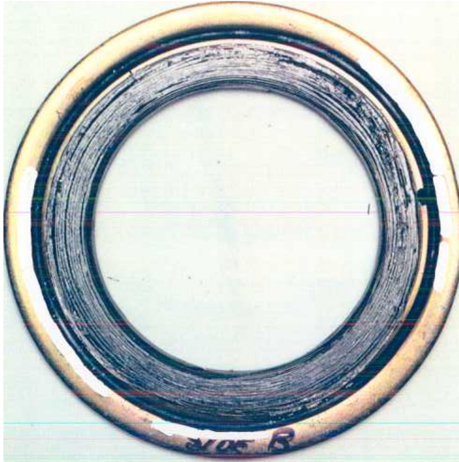
SPIRAL WOUND GASKET AFTER HYDROSTATIC PRESSURE TEST SIDE B
