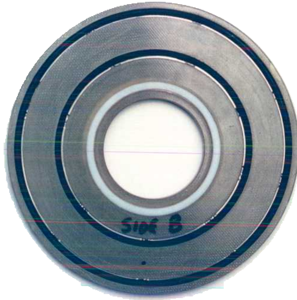
PIKOTEK FLOWLOK VCS GASKET AFTER NITROGEN & HYDROSTATIC PRESSURE TESTS SIDE B
