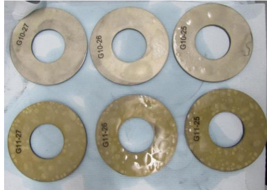
Figure 8: G10/G11 After Sour Gas exposure - 14 days (8)
