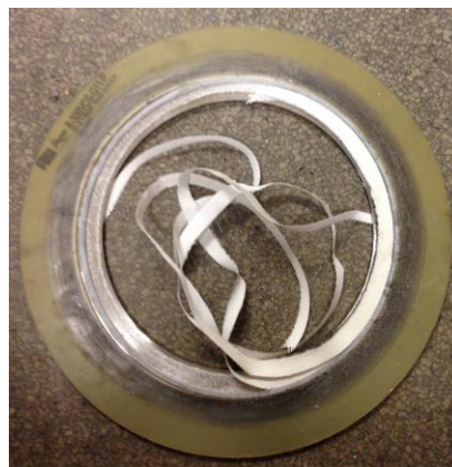
Figure 9: Gasket Exposure to Steam (10)
