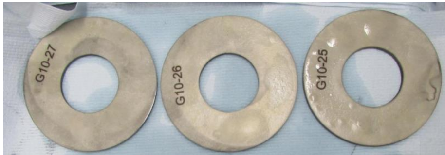
Figure 17: G10 condition after sour fluid exposure at 150°C for 2 weeks
