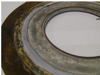
Figure 10: High Temperature exposure of G10 (11)
