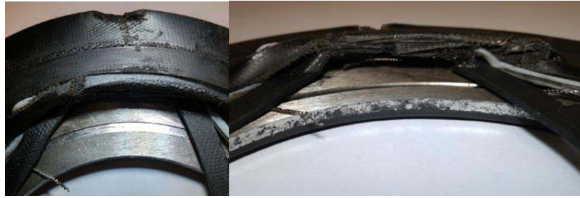
Figure 13: Gasket samples of GRE at High Pressures
