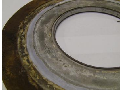
Figure 10: High Temperature exposure of G10 (11)
