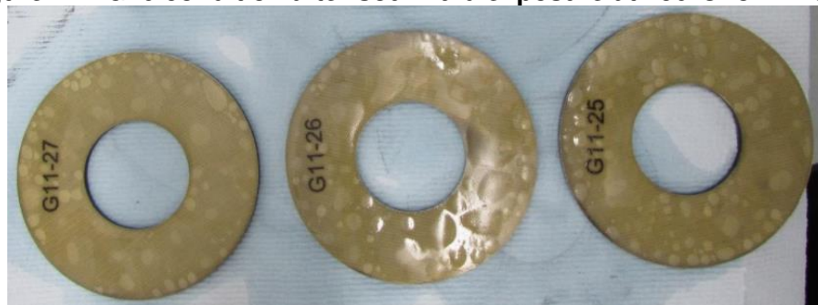
Figure 18: G11 condition after sour fluid exposure at 150°C for 2 weeks
