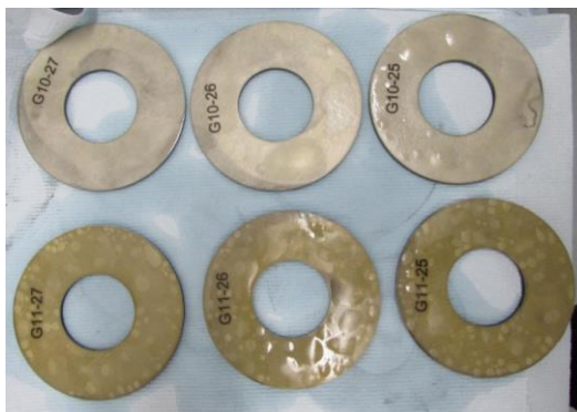
Figure 8: G10/G11 After Sour Gas exposure - 14 days (8)
