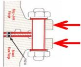
1.4 If the gasket being used has a metal core (VCS®, VCFS®, VCXT®, VCS-ID® & EVOLUTION™), then also test the isolation between each flange and the gasket core.
