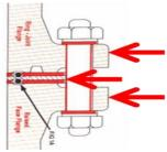
1.5 Test the isolation between one flange and each of the studs.
