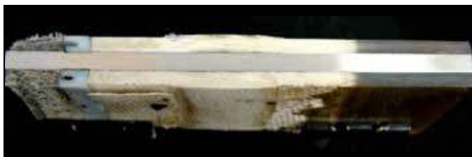
Steam attack on GRE isolation gasket
