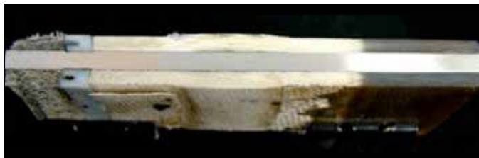
Steam attack on GRE isolation gasket
