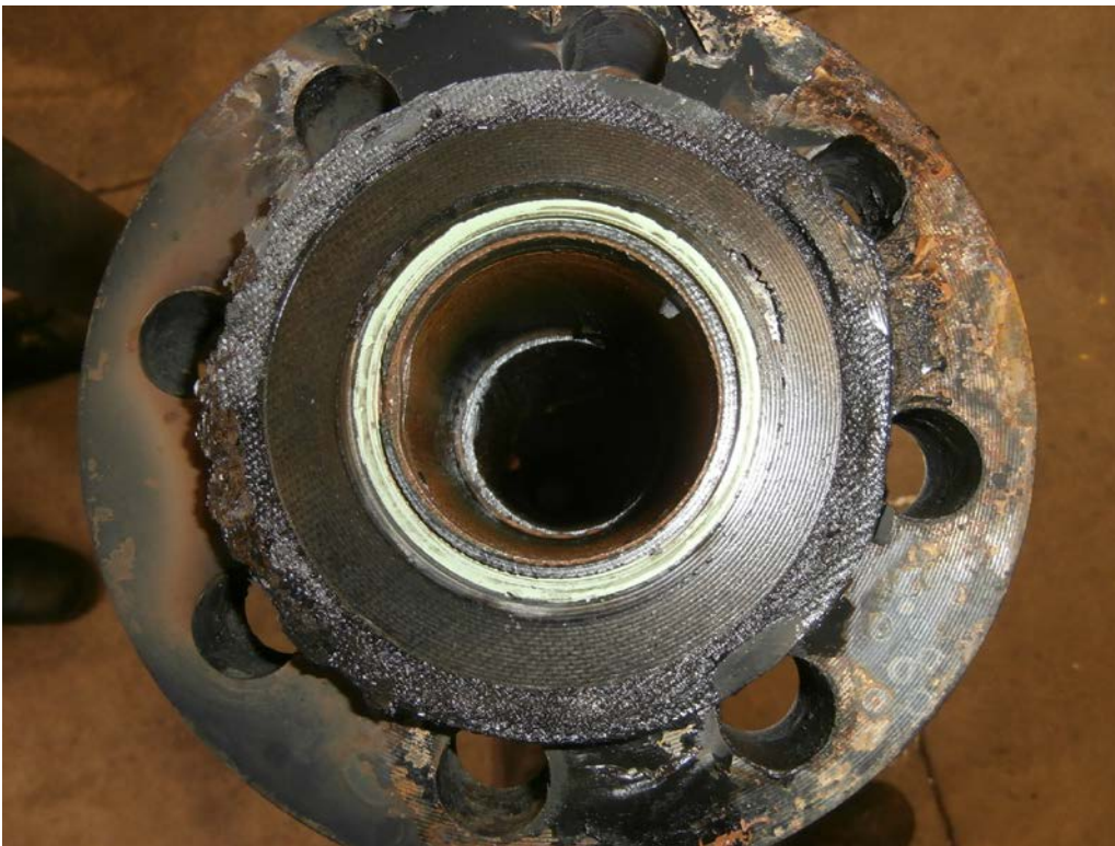
Test Gasket Post-Burn
