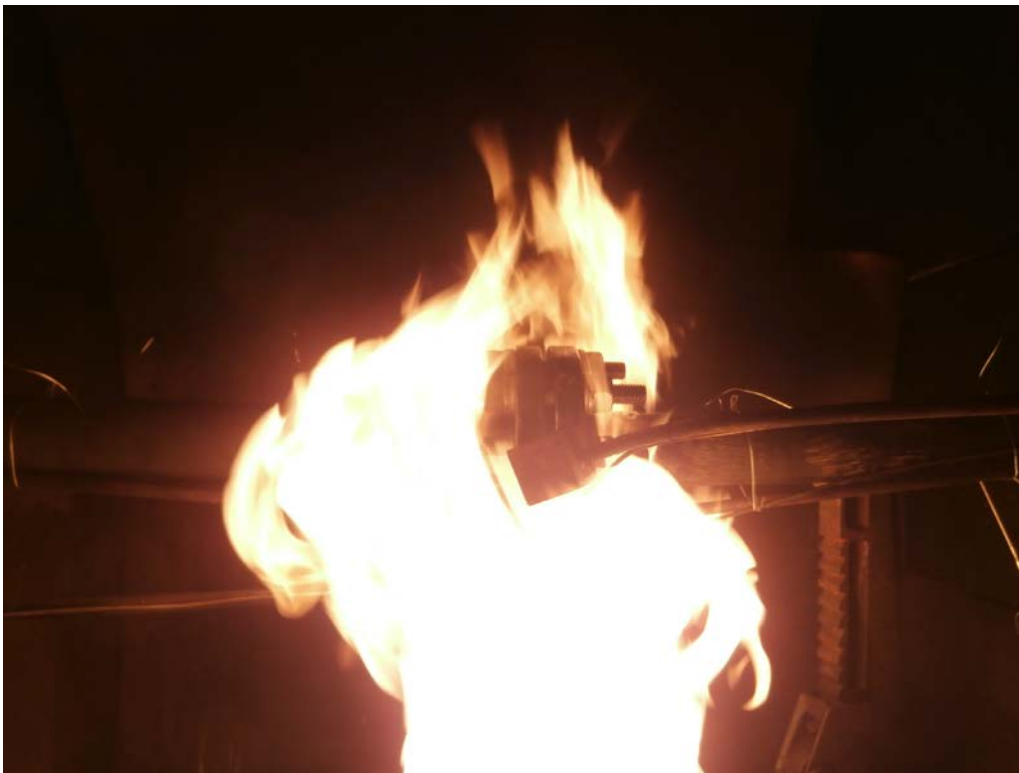
Test Gasket During Burn
