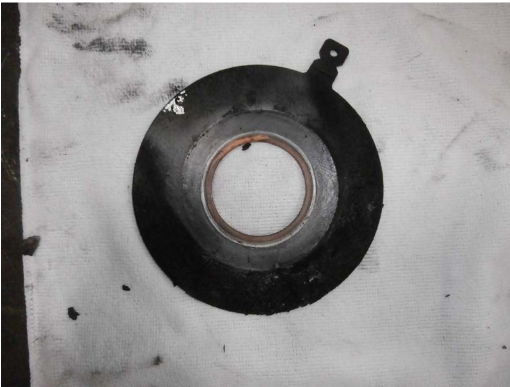
Test Gasket Post-Burn
