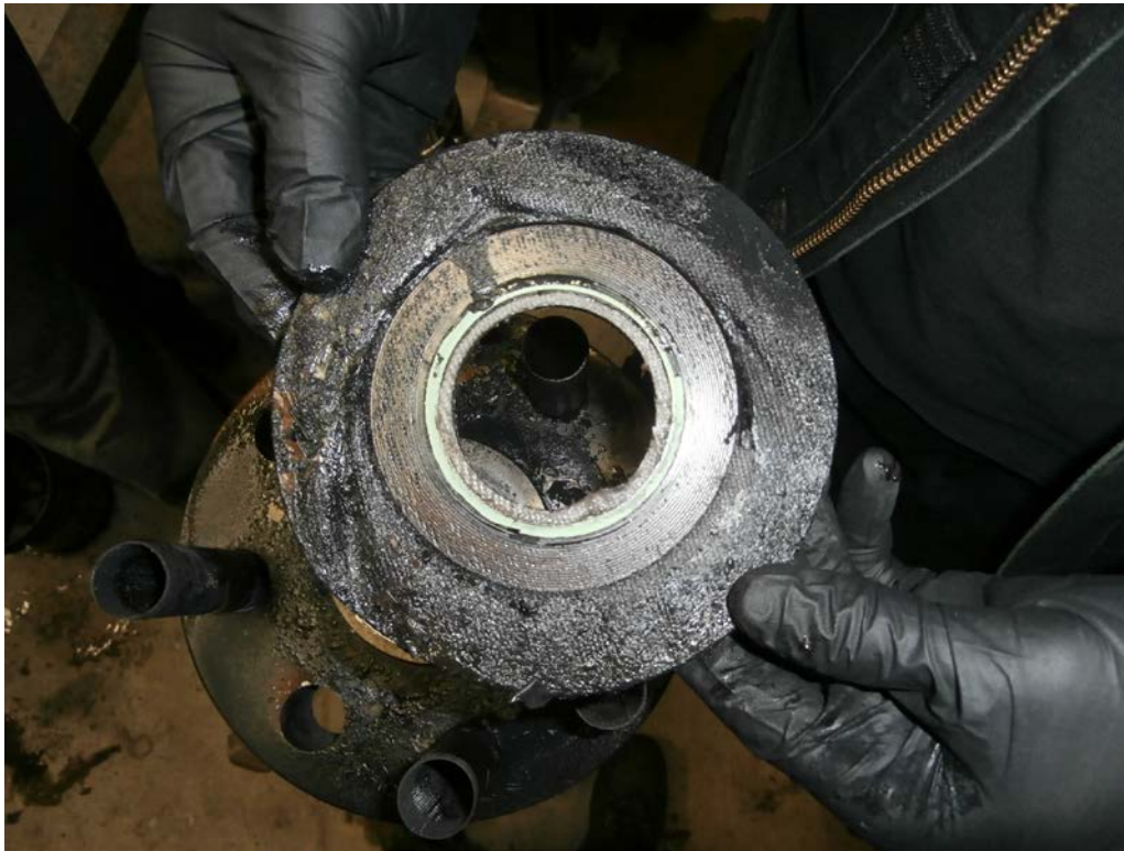
Test Gasket Post-Burn
