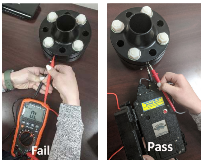
Figure 3. Left: isolation testing using an ohm meter. Right: isolation testing using an RFIT meter.
