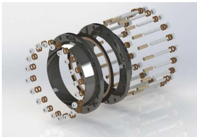
Figure 1. 24 in./600# flange = 193 individual components.
