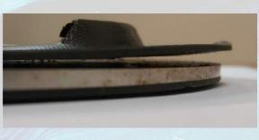
strength of the G10 or G11. High temperature, coupled with improper installation techniques or high pressures, can cause joint blowout.
