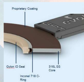
provides a seal that will not be compromised in the event of a fire. The product has been tested to API 6FB fire testing successfully in multiple sizes and classes. The open face of the C-ring also faces towards the media creating a pressure activated seal.
