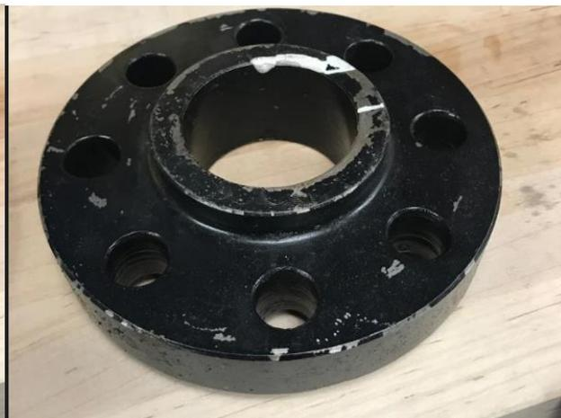
Image 2: Example of a Slip-on Flange
